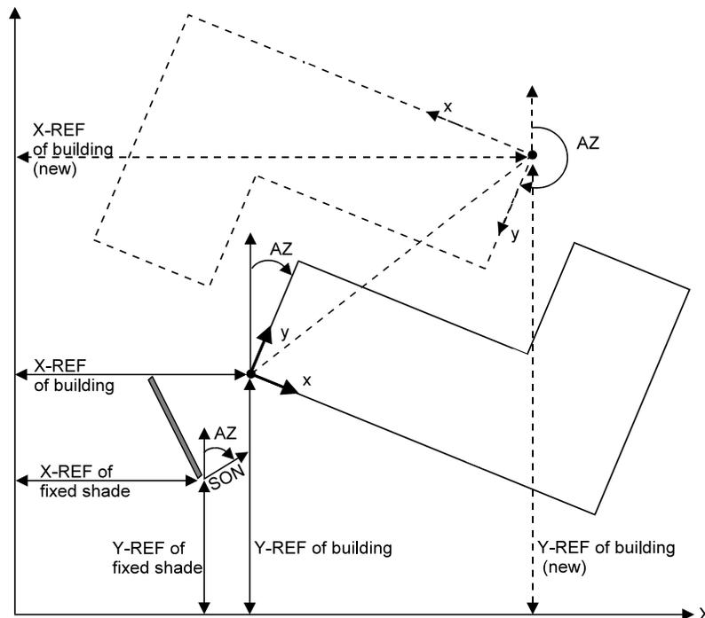
Figure 4 Positioning a building and fixed-shade in the reference coordinate system
