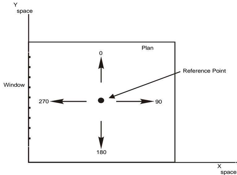
**Figure 23 VIEW-AZIMUTH for four occupant view directions.**
