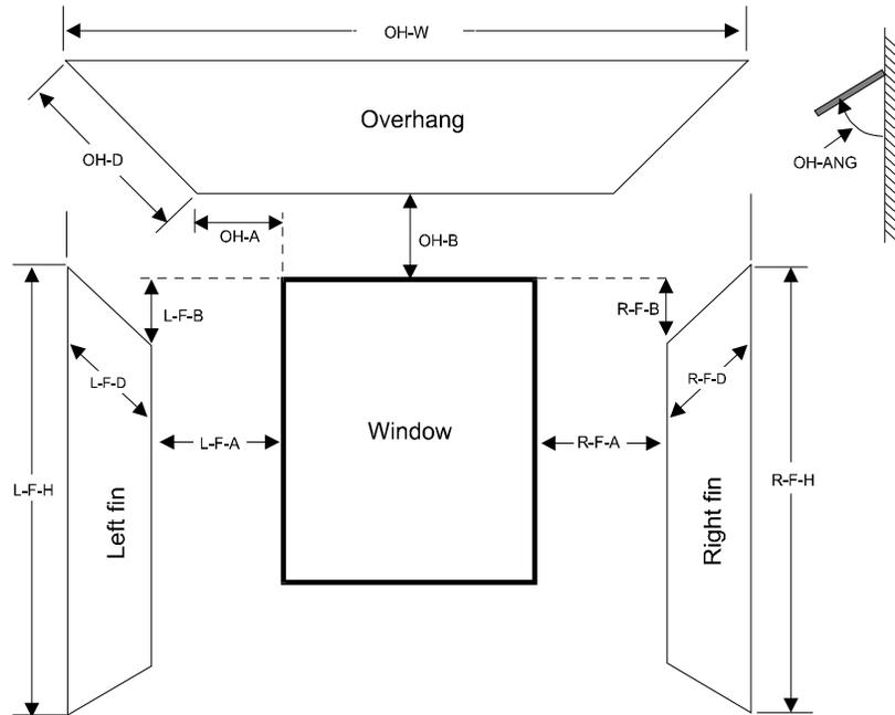
**Figure 26 Positioning of overhang and fins with respect to a window**
