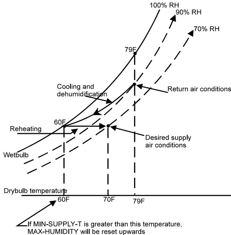
Figure 41 Relationship of MAX-HUMIDITY to COOL-MIN-RESET-T
