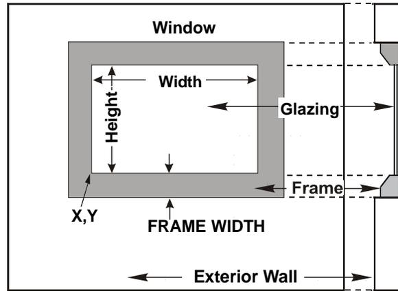
Figure 27 The dimensioning of a window with a frame.
