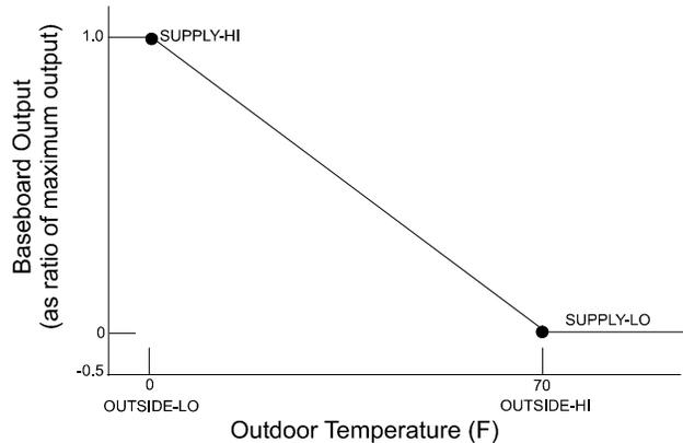
Figure 2 Typical DAY-SCHEDULE-PD:TYPE = RESET-RATIO for baseboard control
