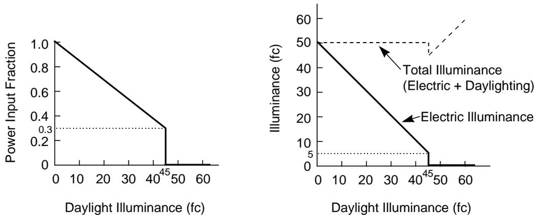
Figure 21 Control action for CONTINUOUS/OFF lighting control.
