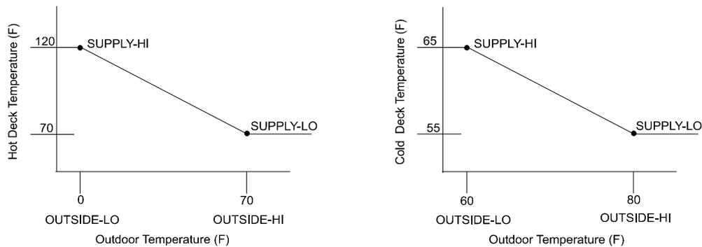
Figure 1 Typical DAY-SCHEDULE-PD:TYPE = RESET-TEMP for deck temperature control
