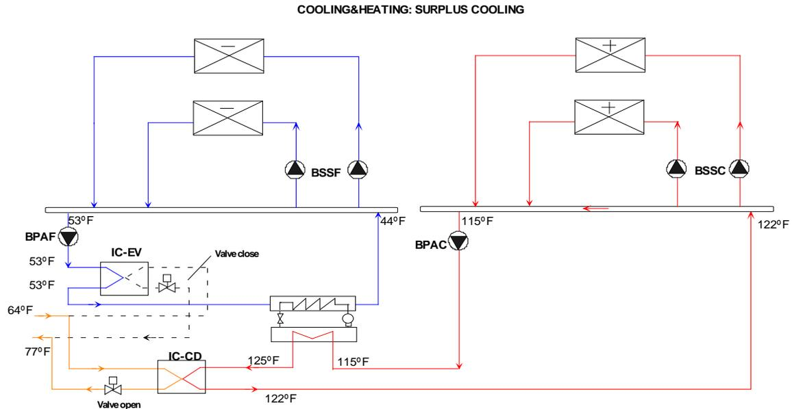
**Figure 33. Loop-to-Loop Heat-Pump
