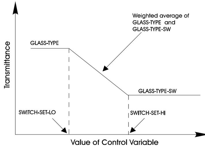
Figure 28 Control Action for Switchable Glazing
