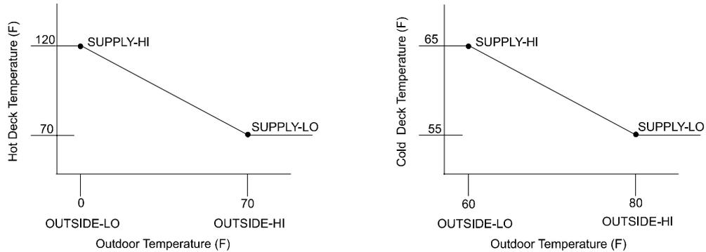
Figure 1 Typical DAY-RESET-SCH for deck temperature control
