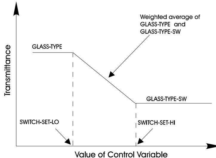
Figure 28 Control Action for Switchable Glazing
