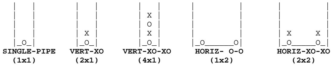
**Figure 35 Pipe arrangements in horizontal wells**
