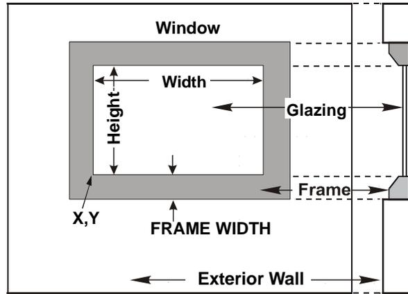
Figure 27 The dimensioning of a window with a frame.
