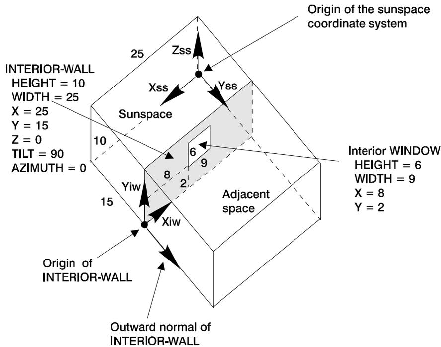
**Figure 8 Positioning an interior-wall in the Space Coordinate System.**
